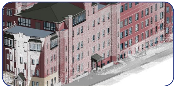
Figure 7: Point cloud data incorporated into Revit to improve the accuracy of the building model
