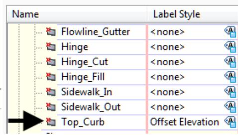
**Figure 10.** Code set styles can be setup to automatically label specific points such as flow line, top of curb, crown, etc.
